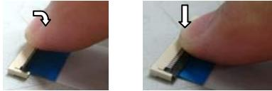
4) : 拔出 FFC 的方法; 依照 1 的方法进行打开掀盖; 在拔出 FFC 时, 请在掀盖完全打开的状态下进行. 万一在掀盖未完全打开的状态下, 拔出 FFC, 重新装入 FFC 时, 请确认触点部位是否有附着物. 4) : pull out FFC method; According to method 1 opens the cover; After removing the FFC, please lift the lid under the fully open position. The lift in one thousand have not completely open state, the FFC is extracted and repack FFC, please make sure the contact area to see if there is attachment.
